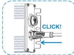
Push connectors together until the lock ring has snapped into place and a click is heard.
