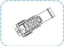
Custom Dimming connection, use a Amphenol X-lok A size connector (AD-03BFFM-QL8DXX(Overmolded with cable) OR AD-03BFFB-QL8AP0(Field installable))
